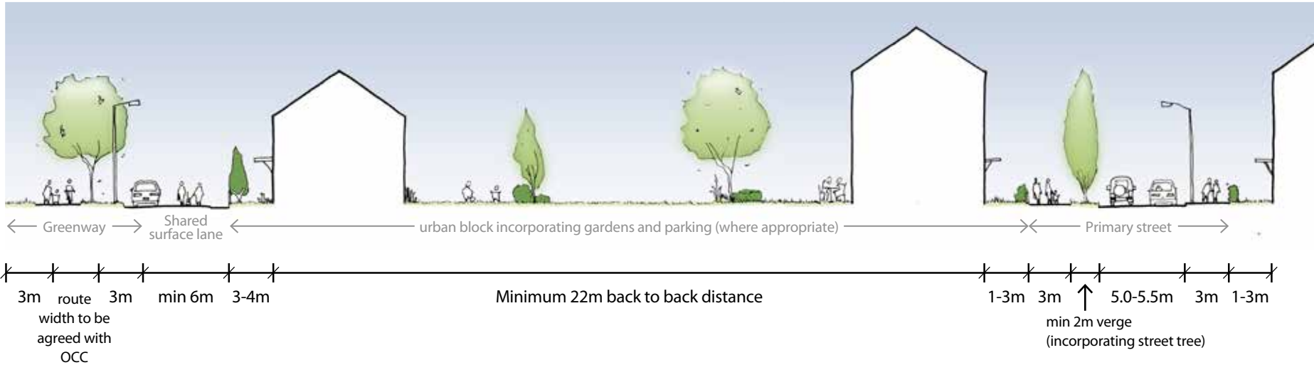
Fig. 18: B-B – indicative, typical central main street cross section (refer to Fig. 17 for section location)
